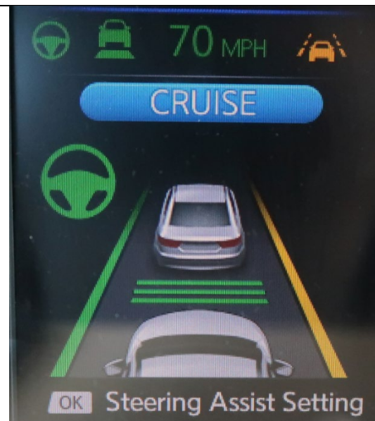
Figure 14: Example steering assist cockpit display on a road with worn pavement markings
