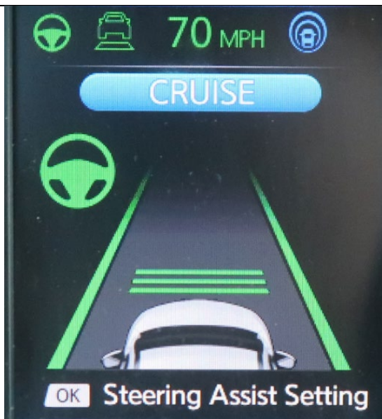
Figure 14: Example steering assist cockpit display on a road with worn pavement markings
