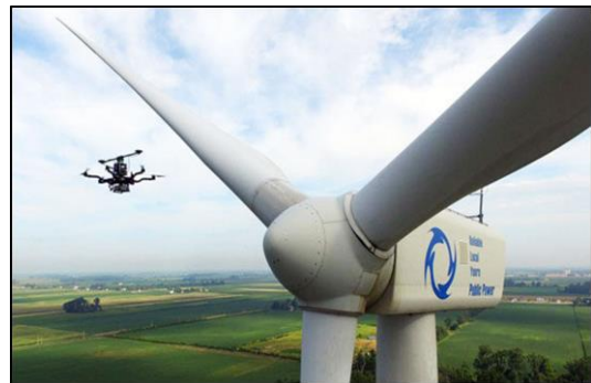
Fig. 3: A SkySpecs drone conducts an automated inspection on a wind turbine at a wind farm.
