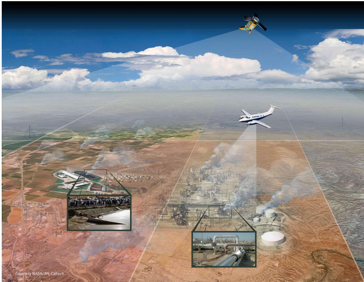
Figure 4 Conceptual view of a “tiered observing system” (system of systems) for methane monitoring including satellites and aircraft that routinely survey large regions and alert teams on the ground to deploy follow-up surface measurements to high emitting facilities for more cost effective and rapid leak detection and repair. [Source: NASA/JPL-Caltech]
