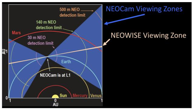
One advantage of NEOCam over ground-based telescopes in searching for NEOs that could potentially hit the Earth is that it scans the sky interior to the orbit of the Earth as well as exterior. Ground-based telescopes only observe at night and so can only search for asteroids when they are outside the Earth's orbit. In five years it will detect 2/3 of "potentially hazardous"
