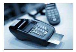
**Figure 3:** Chip-enabled POS terminal with an EMV chip card inserted
