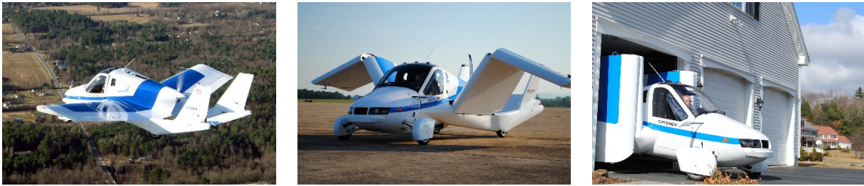
Figure 1: The Terrafugia Transition® in flight, folding its wings, and in a household garage
