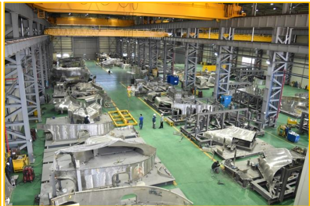
FIG. 12: The 850-ton thermal shield, made up of 600 components that range from a few hundred kilos to approximately 10 tons, is in mass production in Korea.
