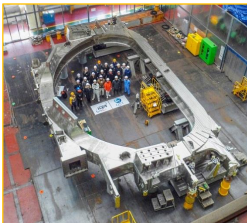
FIG. 9: This toroidal field coil case was manufactured by Mitsubishi Heavy Industries and Hyundai Heavy Industries, in 2 pieces.
