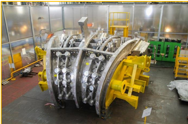
FIG. 11: Korea is nearing completion of the vacuum vessel sector #6. Each sector is made up of four segments. Pictured here is poloidal segment 2.
