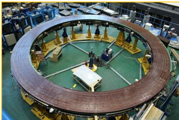
FIG. 13: This double pancake for poloidal field coil #1 in Russia was the first ITER pancake wound following qualification; it has now completed vacuum pressure impregnation to create a rigid assembly.
