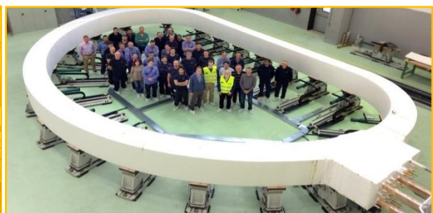
FIG. 6: The first toroidal field coil winding pack – the 110-ton inner core of ITER's TF Coils – was completed in April 2017.
