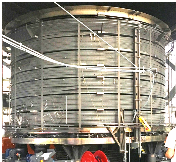
The first of seven magnets for ITER's Central Solenoid following heat treatment to create the solenoid's superconducting material.
