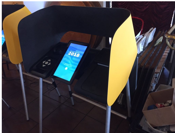
Fig. 2: Los Angeles VSAP prototype, with button-box, touch-screen, and printer.
